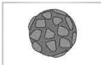
CEMAX adsorbs into small cracks clinker, saturate the charges and reduce the surface energy forces
